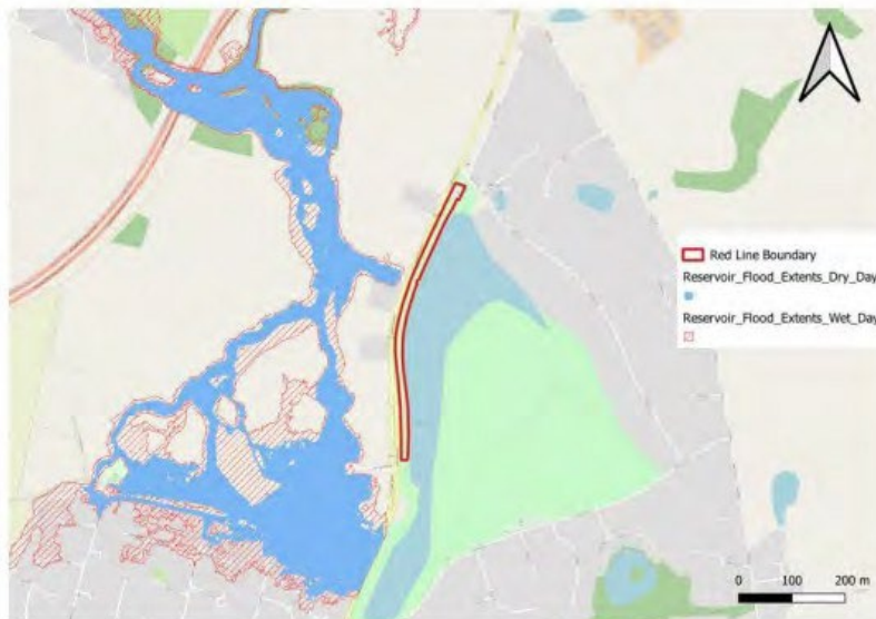
Figure 3-3: Extent of reservoir flood risk surrounding Poynton Lake © Environment Agency copyright and/or database right 2021. All rights reserved. Contains Ordnance Survey data © Crown copyright and database right 2010-2023.
