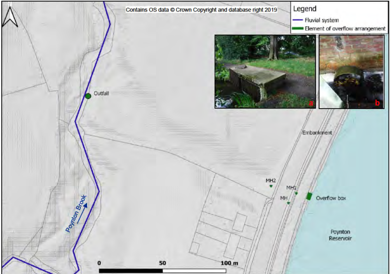
Figure 1-4: Poynton Lake Reservoir Overflow Arrangement, photo inserts show (a) overflow box and (b) internal view of culvert inlet.
